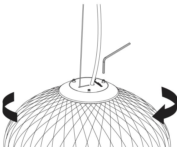
If necessary, the metal fitting on the glass shade can be loosened slightly and turned so the weight can be adjusted in another direction.
