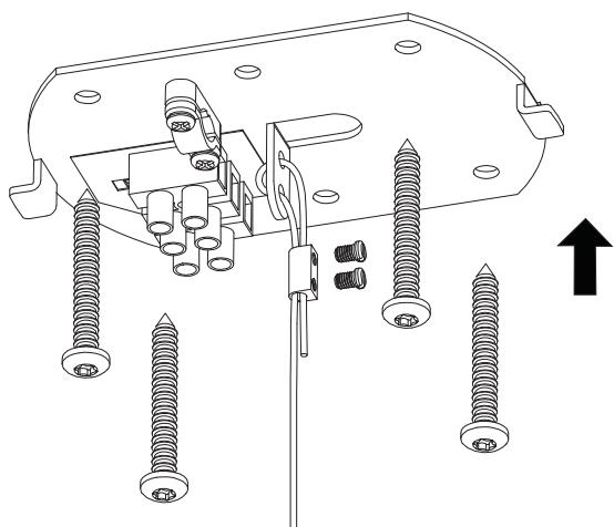
Mount the metal plate securely in the ceiling with screws and appropriate plugs. Fix the safety wire onto the metal plate.
