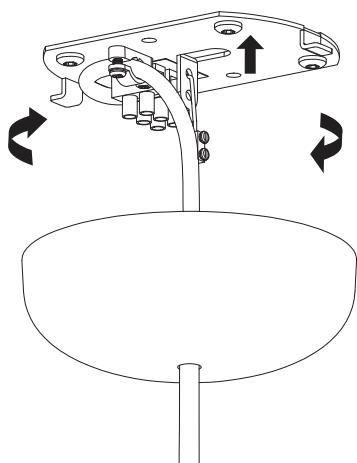
Install the plastic canopy onto the metal plate.
