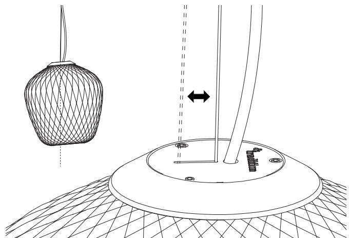
In case the lamp is not hanging straight, the lamp can be balanced by sliding the safety wire to adjust the weight distribution.
