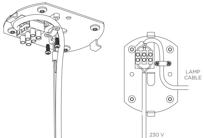
Lead the wires of the lamp cable into the terminal block. Then connect the 230V power supply to the terminal block.
