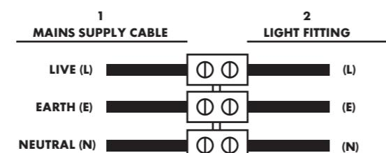
**GB** Connect the fitting and a connector block / junction box to the mains cables as shown in illustration and wiring diagram. Cover cables connected to the connector block with 2 layers of insulation tape.
