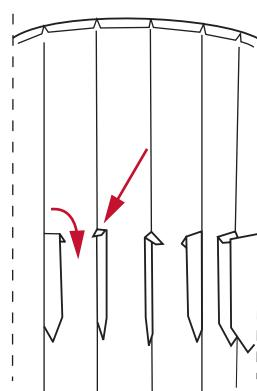
Insert the flaps of the elements into the slits in the central cylinder and cut off the ends on the inside.
