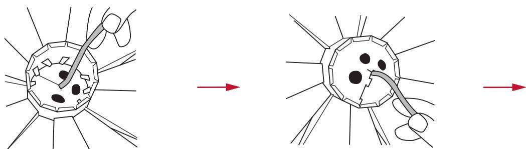
Lower the bulb and bulb socket into the cylinder and press the first hanging element down past the "flaps". Attach the second hanging element to the cable with the point downwards. Lower this into the cylinder, where it will ensure that the lamp hangs straight.
