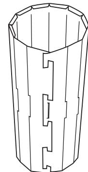
"Snap" the central element together to form a 12-sided cylinder.
