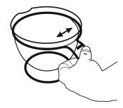
To insert, bend the frame apart at the handle, angle the glass bowl towards the front (spout) and press down on the handle side.
