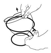
Press the frame wide apart at the handle with thumb and forefinger. (Alternatively, place the jug upside down on the table, pull the handle apart with both hands and lift the frame off the glass jug).
