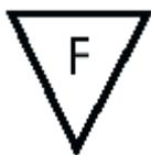
The symbol indicates the suitability of fixtures to be mounted directly on normally inflammable surfaces. Fixtures without the above symbol are only suitable for installatio on non-flammable surfaces
