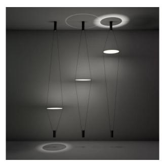
DIRECT AND INDIRECT LIGHT, THANKS TO THE LED LIGHT SOURCES HOLD INSIDE TWO COLORED ALUMINIUM CYLINDRICAL SUPPORTS WHICH ARE AT THE ENDPOINT OF THE TWICE POWER CABLES. ONE IS FOR THE CEILING CONNECTION, THE OTHER ONE IS USED AS A COUNTER-WEIGHT. THE LIGHT IS REFLECTED ON A SWIVEL DISK IN A WHITE OPAL METHACRYLATE MATERIAL WHICH SPACES AND SLIDES ALONG TWO CABLES, TO CREATE DIFFERENT LIGHT EFFECTS. INFERIOR CYLINDRICAL SUPPORT WITH A CABLE AND AN ELECTRONIC DRIVER ON THE PLUG.
